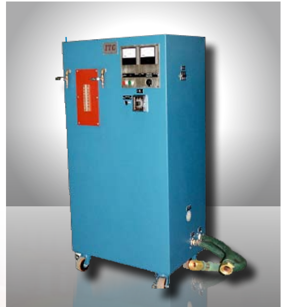
Shown with the “workhead” transformer mounted through the front for connection to the heating coils
